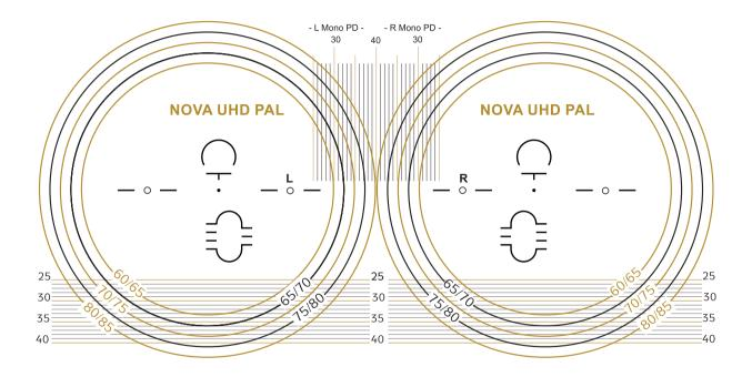
Fitting cross is located 4mm above lens Prism Reference Point
